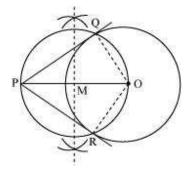
$\angle$  PQO is an angle in the semi-circle. We know that angle in a semi-circle is a right angle.
